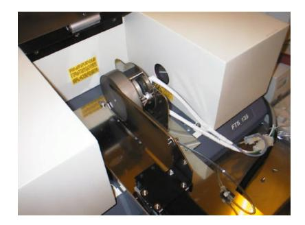
Fig.1. External view of the FT-IR measurement tool with wafer transport and *in situ* bake system.
